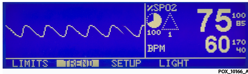
Figure 96. PLETH Display with SRC-MAX decrease in modulation
