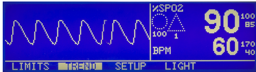
Figure 94. PLETH Display with SRC-MAX increase in %SpO 2 of 90 with modulation
