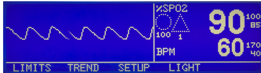
Figure 101. PLETH Display with SRC-MAX increase in %SpO2 of 90 with high light condition
