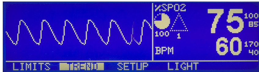
Figure 95. PLETH Display with SRC-MAX increase in %SpO 2 of 75 with modulation
