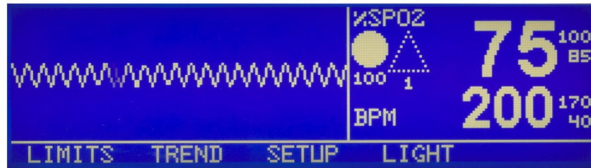
Figure 99. PLETH Display with SRC-MAX increase to 200 BPM with high light condition
