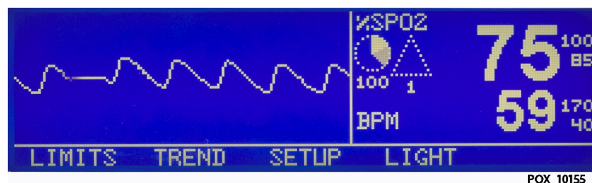
Figure 97. PLETH Display with SRC-MAX tester-generated waveform
