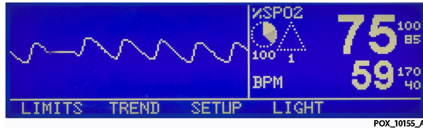
Figure 90. PLETH Display with SRC-MAX tester-generated waveform
