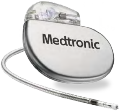
Traditional single-chamber pacemaker and lead
